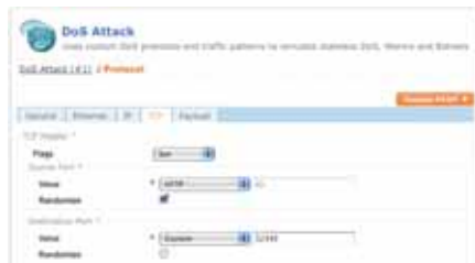
Figure-1. Intuitive GUI helps users customize the type, pattern, rate and duration of a simulated DoS attack via simple XML templates.
