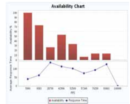
Figure-3. Interactive charts and reports enable users to visualize the negative impact on system response time and service availability under a DoS attack.
