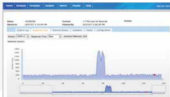
Figure 1: An example of a response-time spike (soft fault) and a subsequent system crash (hard fault), where the red dot denotes the crash.
